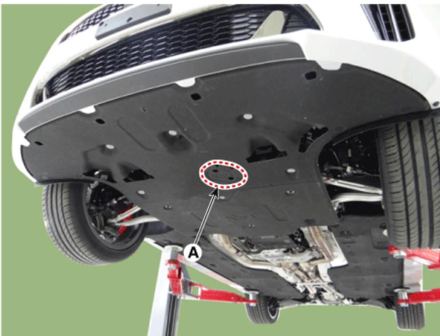
(2) Remove the oil filter cap (A).
